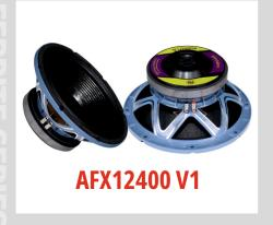
400-800W **Power Rating Nominal Impedance** 8 Ohm Frame Cast Aluminium **Voice Coil** 3" Size/ Net wt. 12"/ 6.9 Kgs 190x90x20 mm **Magnet Size** Frequency 50 Hz - 3.5 Khz
