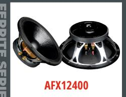
400W **Power Rating** Nominal Impedance 8 Ohm Frame Cast Aluminium **Voice Coil**
